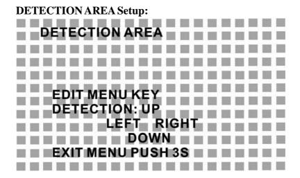
Detection Block Setup: Press MENU button to enable or disable a single cell configuration setting Use up and down keys to move around or to end the setting mode. Press MENU button for 3 seconds to leave the setting page.
